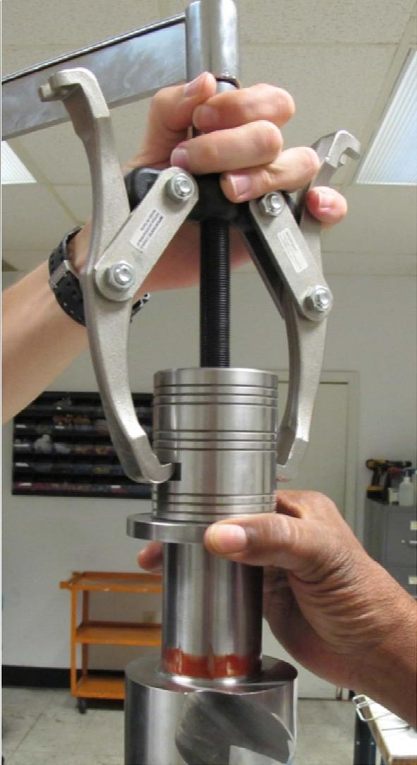
Use a gear puller to remove the shoe.
