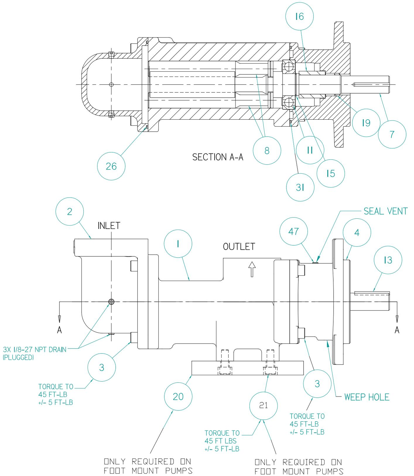
Fig 5 - Steel Pump Assembly
