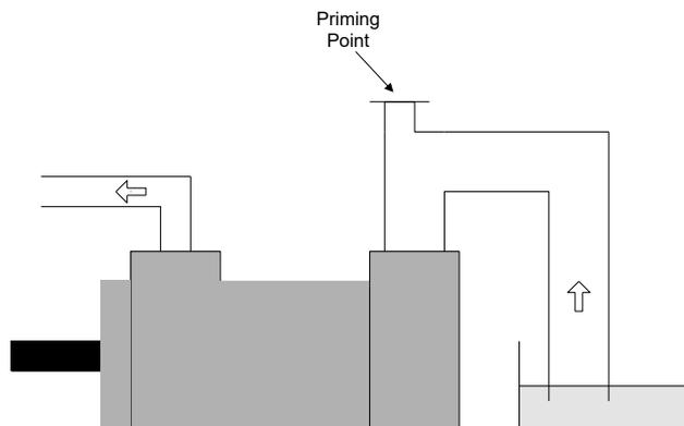
**Figure 12 – Priming Pump Using Priming Port**
