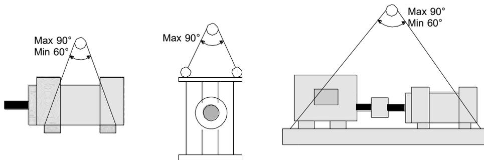
**Figure 1 – Lifting Pumps and Pump/Driver Assemblies**
